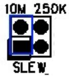
10M: Disable slew rate limit feature. Maximum communication speed for this mode is at 921.6Kbps.
